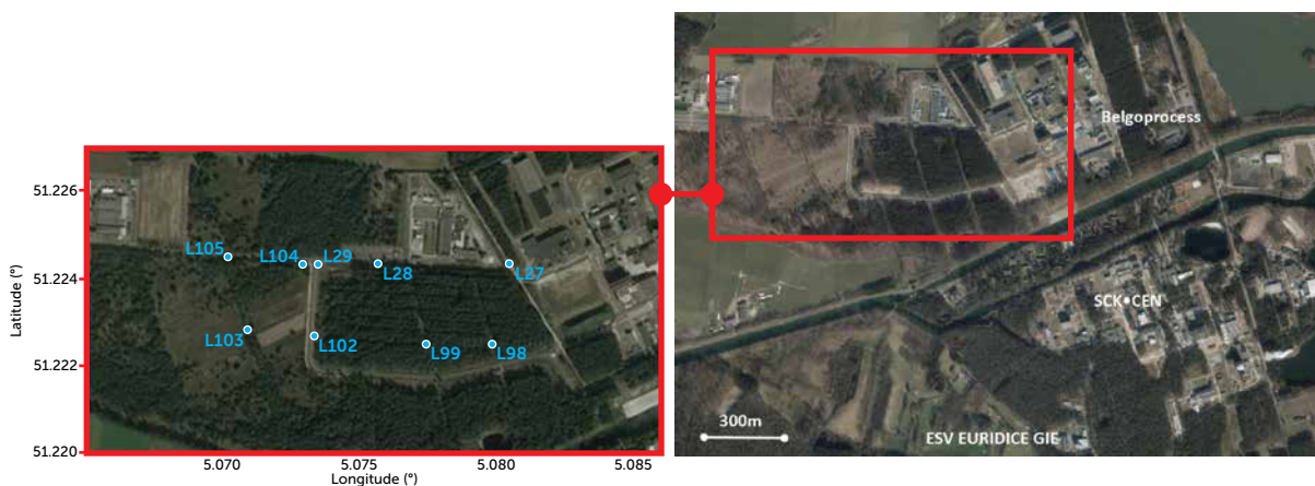
Figure 32 - Location of the nine piezometers used for point dilution tests, part of the additional experimental programme for validation of the hydrogeological models
