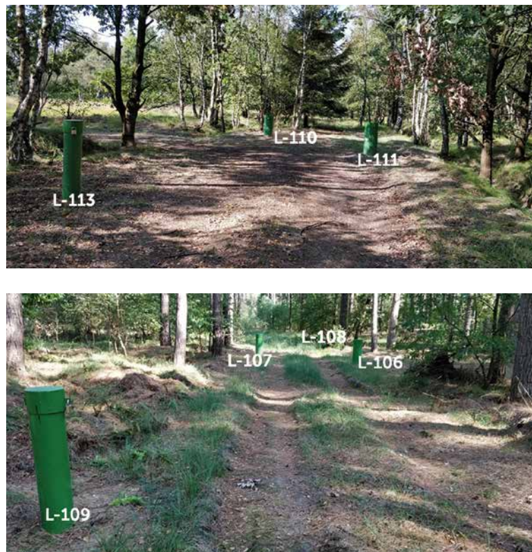
Figure 34 – Upper picture: three of the four piezometers in the "West" cluster; L-110 and L-111 are the pumping wells and L-113 and L-112 (not shown) are the observation wells. Lower picture: "East" cluster with pumping wells L-106 and L-107 and observations wells L-108 and L-109.
