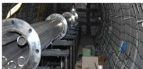
Figure 3 - Cross-section of the central tube and view of the primary heating system
