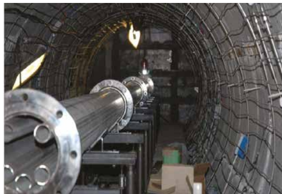
Figure 4 – Cross-section of the central tube and view of the primary heating system
