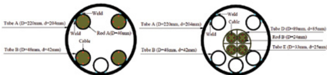
Figure 5 - Eight heater assemblies of the secondary heater to be installed in the central tube
