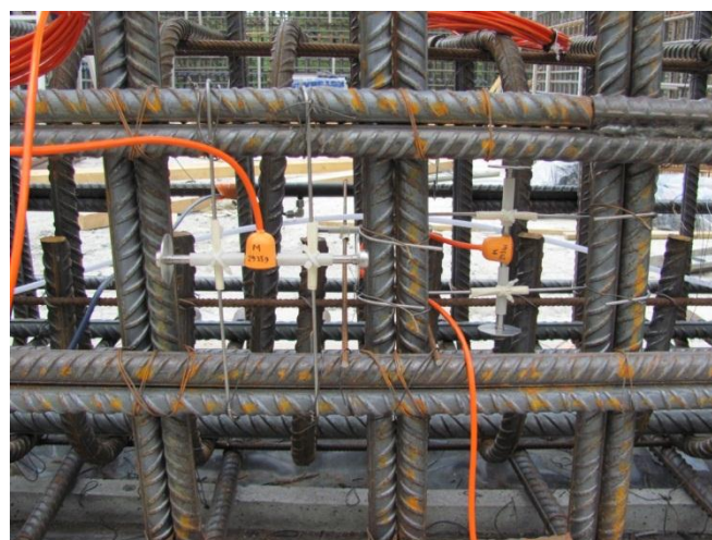
Figure 26 Example of instrumentation placed in the test set-up
