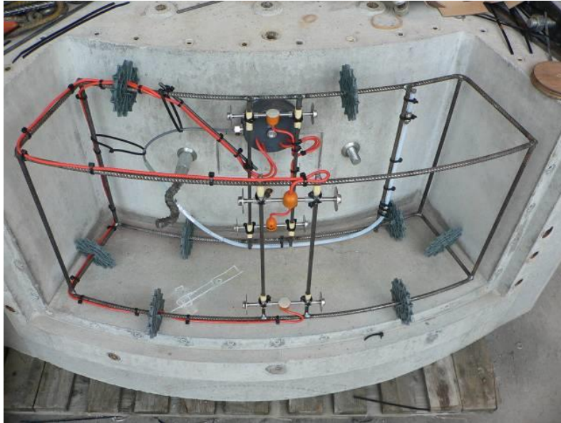
Figure 14 - Support case placed in the segment mould for the installation of the strain gauges
